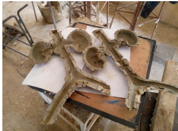
Figure 1. Casted mold (right and left side).
