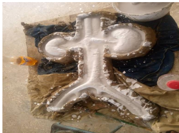
Figure 2. Casting stage (mold casting with P.O.P).
